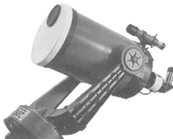
Illustration 8: Celestron C-8 with DayStar Filter and Off Axis Prefilter attached.
